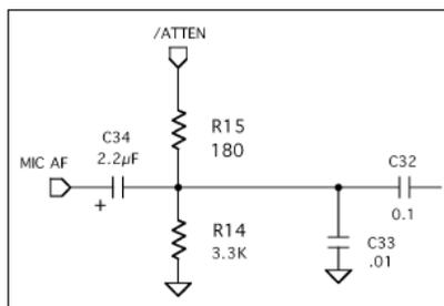
The K2 feeds the the compressor chip directly, not using any preamplifier. Regarding the KSB2 Manual the microphone should give 100mVpp (peak to peak) The Microphone signal is attenuated by R14/R15 using R15 in Menue settig SSBA=1 parallel to %14. If you increase the value of R14, you can use the microphon sensitivity. Using an MH2 Mike, we found 3,3 kOhm instead of the original 1k was the best value.
