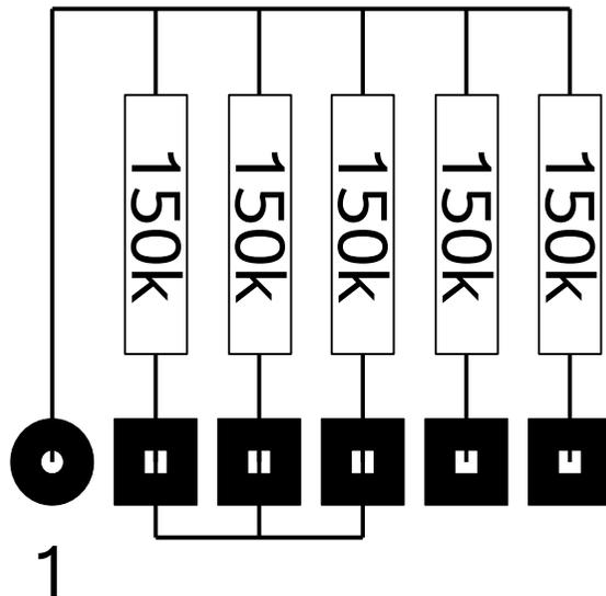
[ ] Install 5 150 k Resistors instead of the Resistor array, as shown in th edrawing. Connect PIN 2,3 and 4 on the solder side of the PCB.
